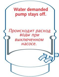
The Zilmet HYDRO-PRO tank leaves the factory already tested and pre-pressurized. Air and water do not mix eliminating any possibility of "waterlogging" through loss of air to the system water; no corrosion possibility.
